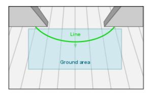
When configuring, remember to activate ground inclination (**Tilt**) in X or Y and check that the found inclination by the sensor in automatic mode corresponds well by displaying the grid. When the parameters are satisfactory, it is recommended to return to **manual mode** by copying the automatic mode values (see Ground Definition).
