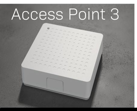
Dual band (2.4GHz + 868/915 MHz) PoE/ USB-C powered access point Your Smart Building Foundation
